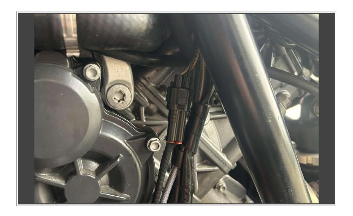
**Position gear sensor** Left side of the motor, below the pinion.
